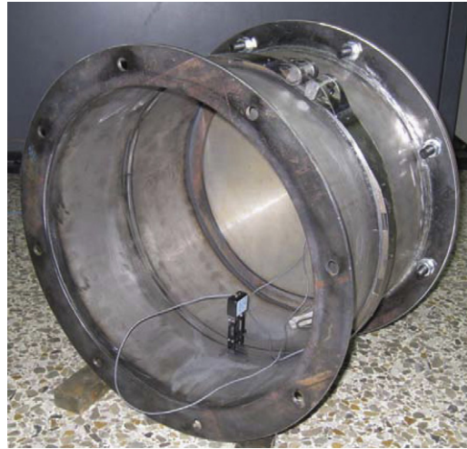
Fig. 9. Configuration of the test specimen with the attachment of the extensometer.
